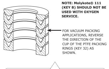
Figure 29 Single Style Packing Installation Diagram
