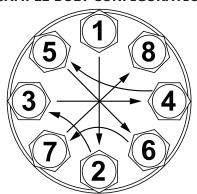
Figure 27 Bolt Tightening Pattern Diagram
