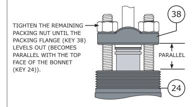
Figure 30 Double PTFE V-Ring Packing Tightening Diagram
