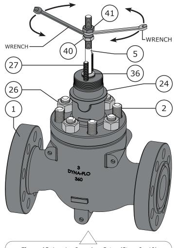
Figure 18 Lapping Procedure Setup (Steps 8 - 10)
