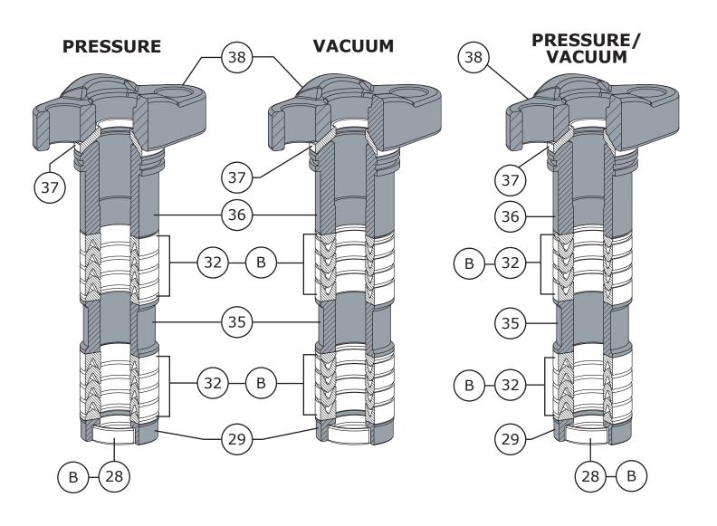
Figure 33 Double PTFE Packing Diagrams
