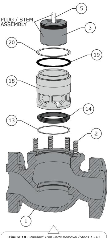
**Figure 10** Standard Trim Parts Removal (Steps 1 - 6)
