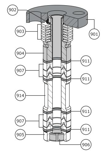
Figure 31 Graphite Packing Arrangement Diagram
