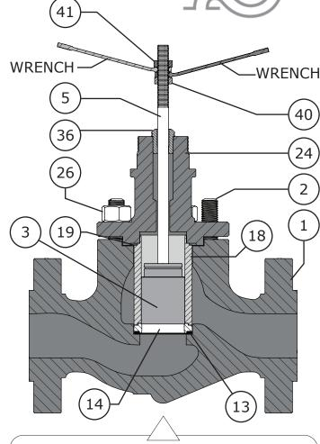
**Figure 16** Lapping Procedure Setup (Steps 1 - 8)
