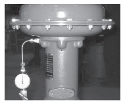
Figure 3 Needle Valve with Gauge setup
