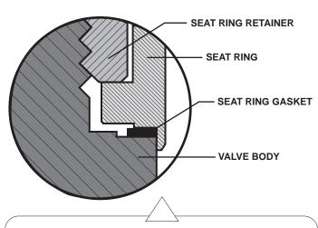
Figure 5 Detail B - Seat Ring Gasket
