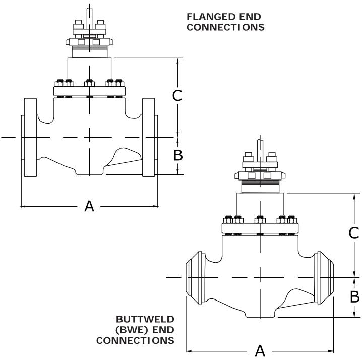
Figure 2 Typical Valve Dimension Diagram
