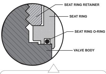
Figure 4 Detail B - Seat Ring O-Ring
