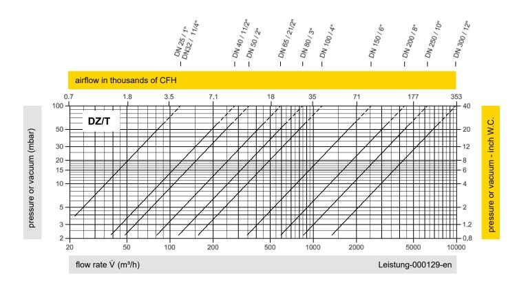
The flow capacity charts have been determined with a calibrated and TÜV certified flow capacity test rig. Volume flow  $\dot{V}$  in (m³/h) and CFH refer to the standard reference conditions of air in ISO 6358 (20°C, 1bar). For conversion to other densities and temperatures, refer to Sec. 1: "Technical Fundamentals."
