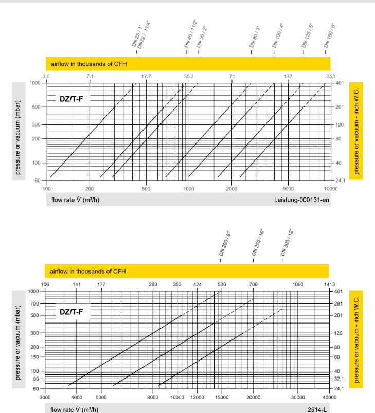
The flow capacity charts have been determined with a calibrated and  $T\ddot{U}V$  certified flow capacity test rig. Volume flow  $\dot{V}$  in (m³/h) and CFH refer to the standard reference conditions of air in ISO 6358 (20°C, 1bar). For conversion to other densities and temperatures, refer to Sec. 1: "Technical Fundamentals."
