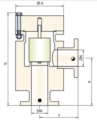
Tank connection for pressure relief function
