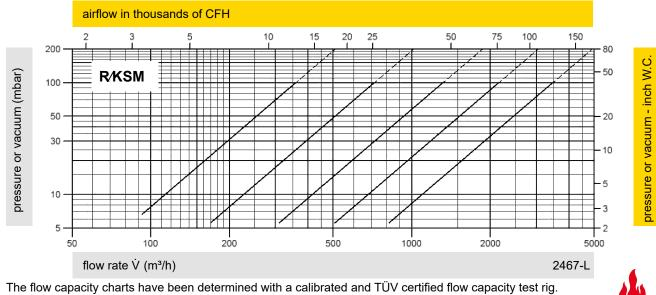
Volume flow V in (m<sup>3</sup>/h) and CFH refer to the standard reference conditions of air in ISO 6358 (20°C, 1bar). For conversion to other densities and temperatures, refer to Sec. 1: "Technical Fundamentals."
