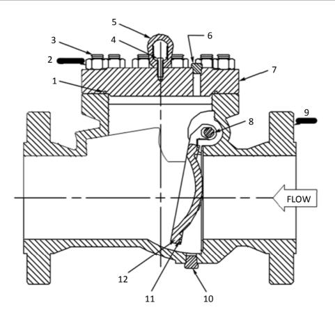
Figure 1 - Integral Seat Swing Check
